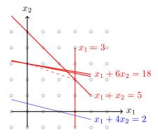
Figure 5.2: Cutting plane approach for MILP.
