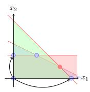
Figure 2.6: The search process of the simplex.
